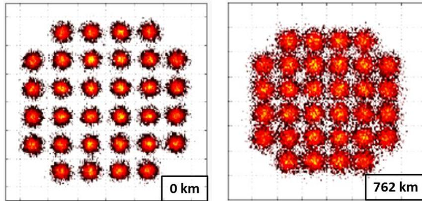
The figure shows an example of a 32QAM WDM channel before and after transmission over 762 km; (The transmission capacity of the link is proportional to the number of dots.)
