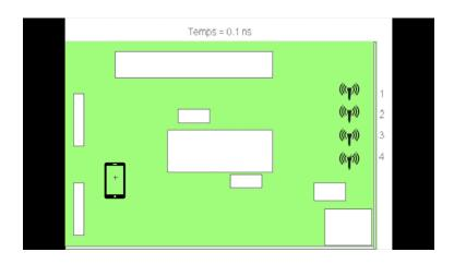
2. Focusing phase: Base Station uses the measured channel, exploits uplink-downlink channel reciprocity and computes the beamformer
