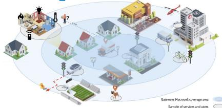
I LoRaWAN Gateway per Km2 Sometimes Coverage problems and some packet lost Deployment messy Battery life (3- 10 years) AES security Geolocalization basically over GPS and WiFi, BLE Sniffing
